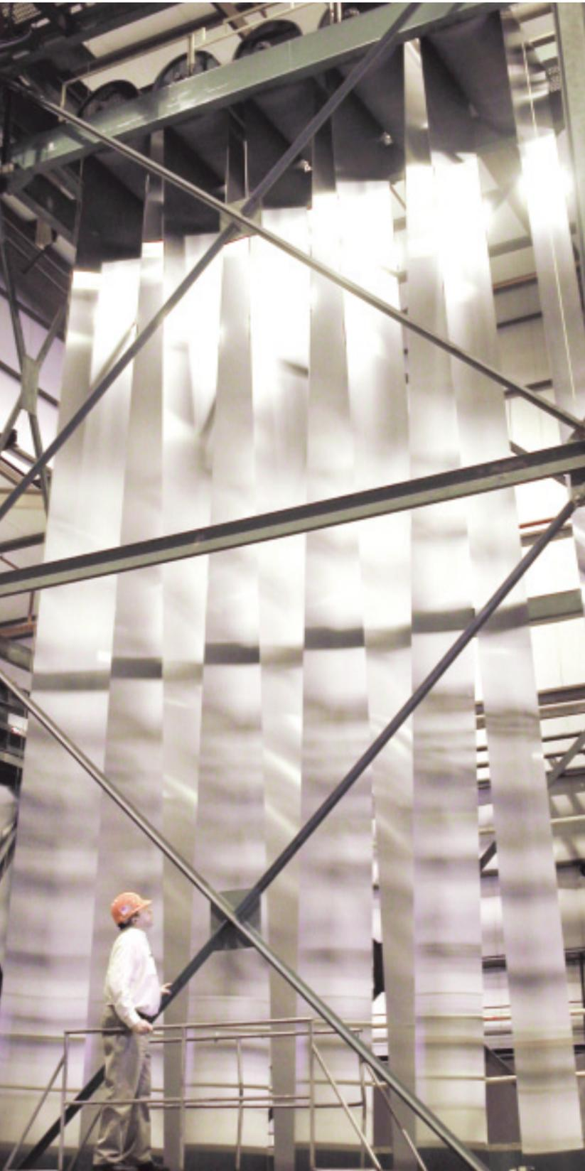
To produce pre-painted aluminum coil, Alcoa Mill Products uses a high speed process (called coil coating) to apply paint and other special coatings to one or both sides of a continuous coil of flat rolled aluminum. In this very efficient process, the speed of the coating line can range up to 400 feet per minute.
