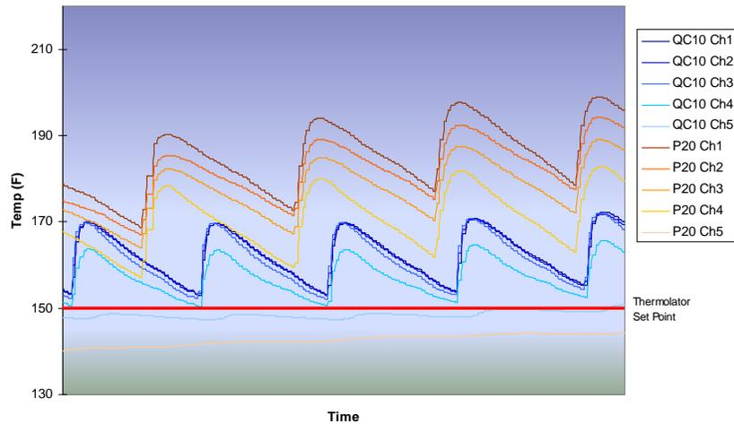
**Trial Three - Two materials, 1 amorphous and 1 semi-crystalline, 3 mm unit molds of QC-10-and P20, pack and hold**
