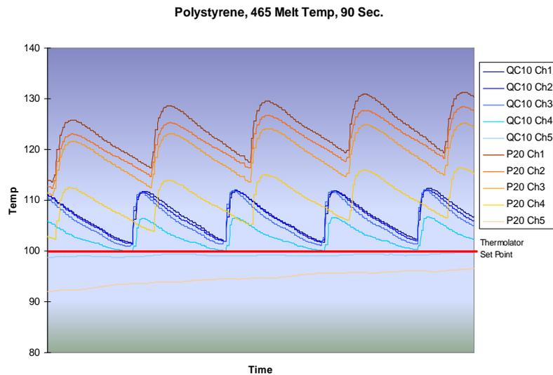
part to get the best achievable result. Cycle was established when the sucker pin pulled the sprue clean and the part was cool enough to eject. Cycle time and mold temperatures were documented for each tool running at least 25 parts at cycle.
