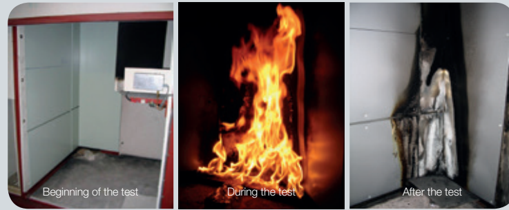
On the test above on our aluminium composite panels we observe that the impact of the fire is confined to the initial heat source because the aluminium hindered the fire to spread further.
