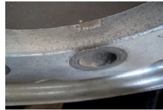
Corrosion wheel nut area and inside bore
