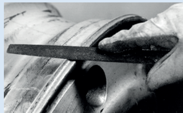
A file can be used very effectively to remove the sharp edge.
