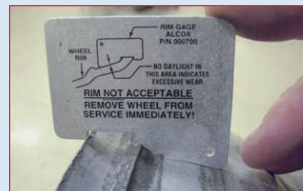
NOT acceptable rim flange wear
