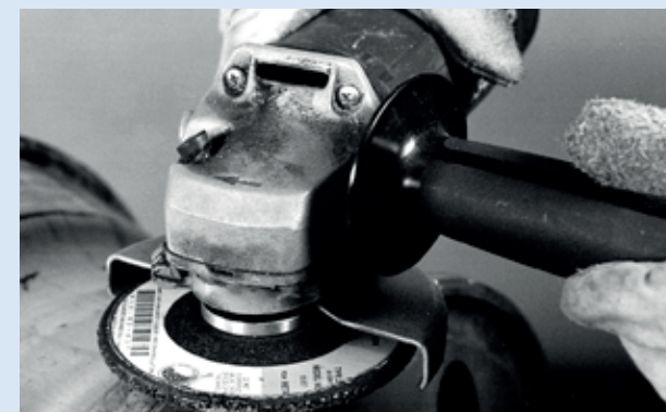
Use die grinder to remove metal. Do not gouge the wheel.
