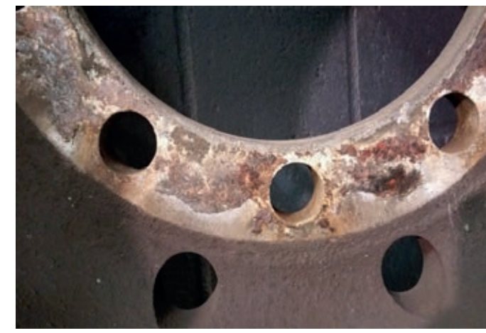
Corrosion mating faces of wheel
