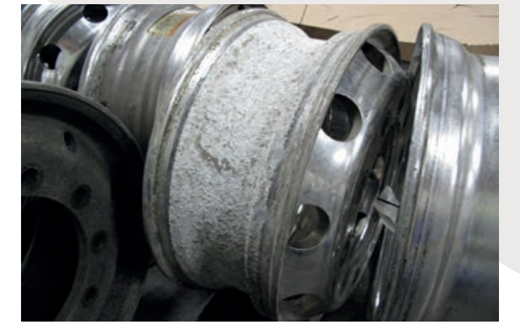
Corrosion caused by liquid tyre balancers or sealants
