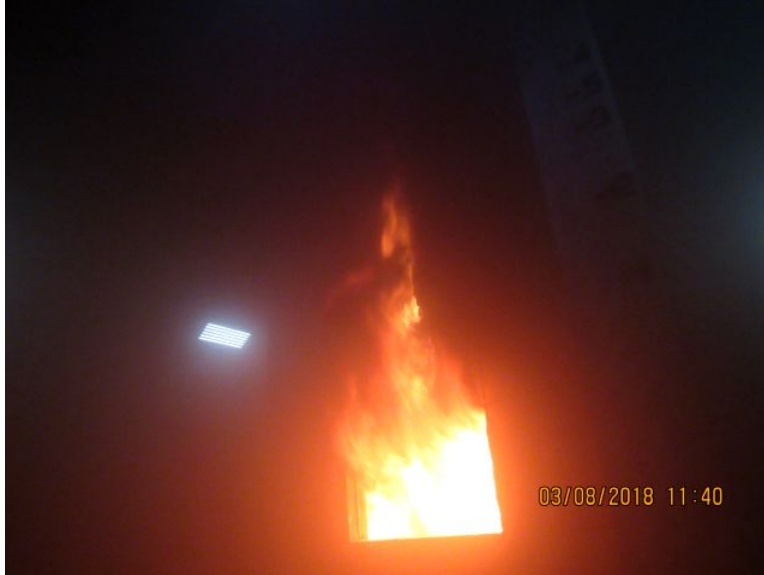
Photo No. 33 Panels Burning 1 m Above Opening
