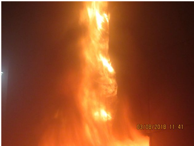
Photo No. 34 Panels Burning 2 m Above Opening
