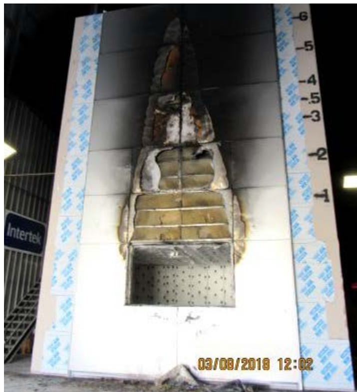
Photo No. 38 Photo of System Approximately 7 min After Furnace Off
