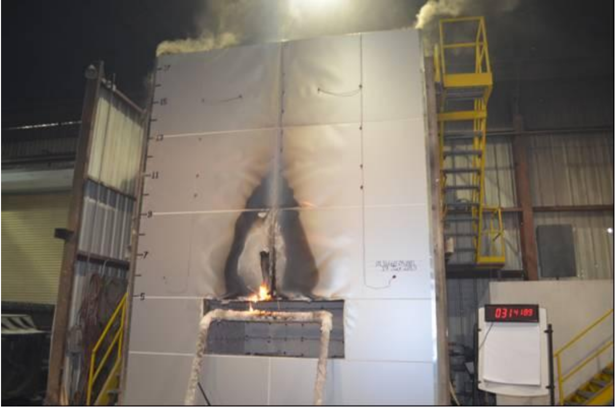
Figure B-17. Exterior View of Wall Assembly during Observation Period. Residual Flaming at Header.
