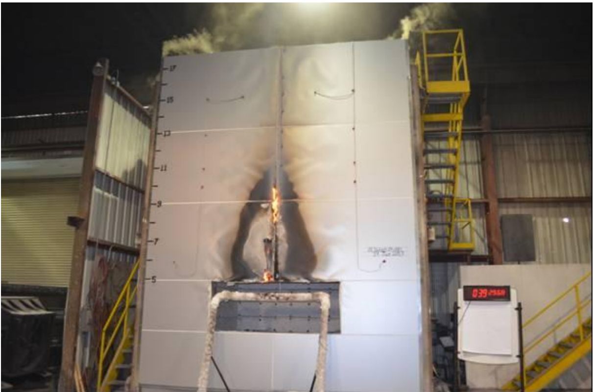
Figure B-18. Exterior View of Wall Assembly at End of Observation Period. Residual Flaming at Header and Central Vertical Panel Joint.
