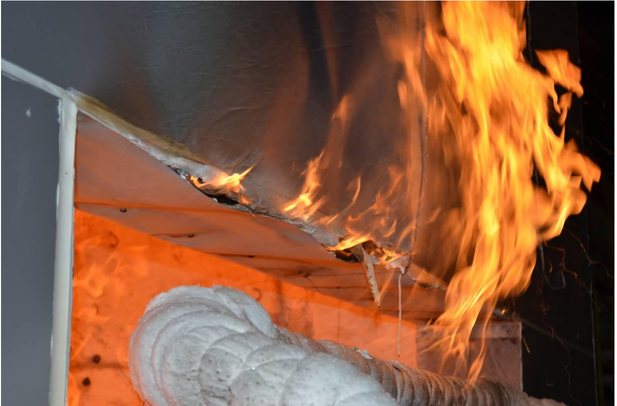
Figure B-11. Flaming from Panel Joint at Window Header Flashing at 13 min.
