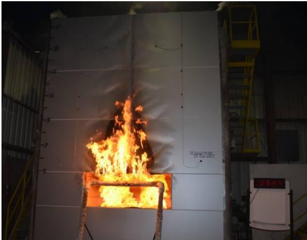
Figure B-14. Exterior View of Wall Assembly at 25 min 8 s.
