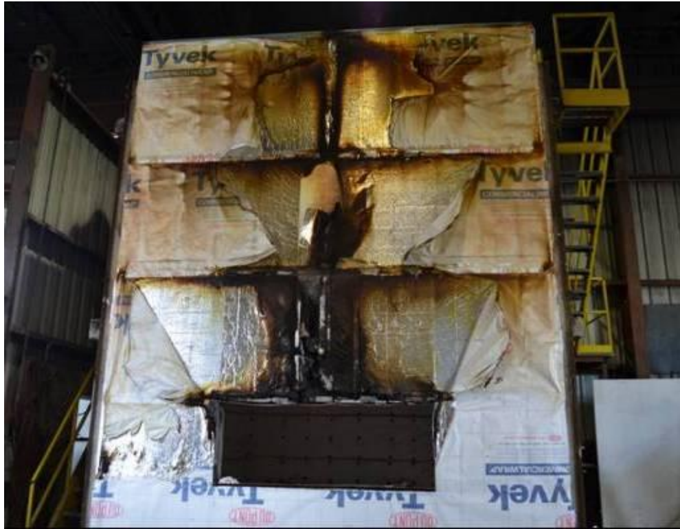
Figure B-21. Post-Test Assembly Dissection: Exterior Face of Polyisocyanurate Insulation following Test.
