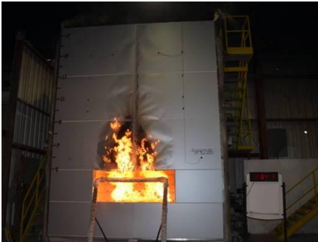
Figure B-12. Exterior View of Wall Assembly at 16 min 41 s.
