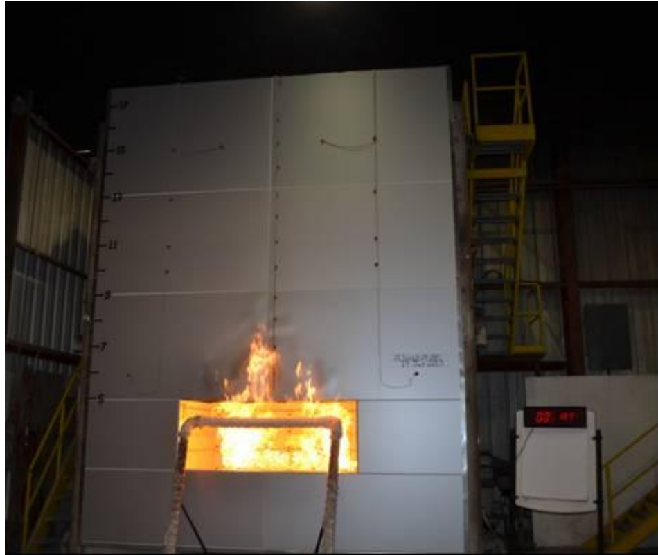
Figure B-9. Exterior View of Wall Assembly at 5 min 18 s.
