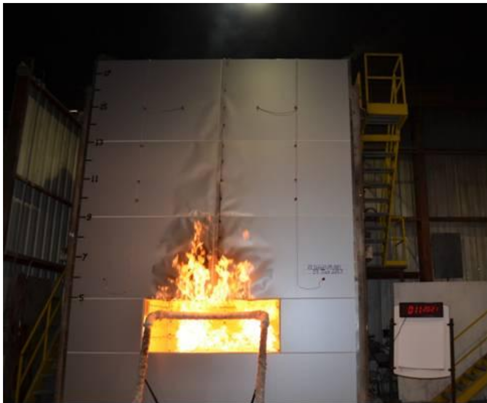
Figure B-10. Exterior View of Wall Assembly at 11 min 20 s.
