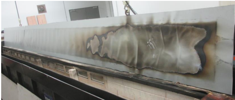
Photo No. 5 Exposed Surface of the Test Specimen (Post-test)
