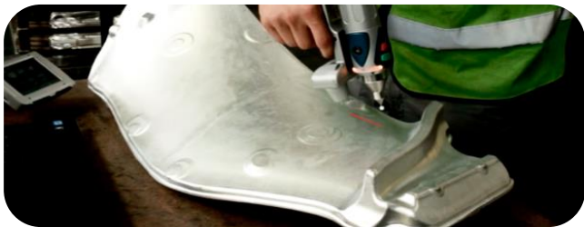
Inspection of a forged front fan blade for aero engine
