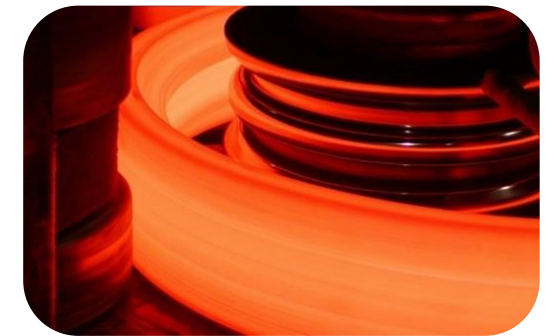
Production of titanium rings for aero engines
