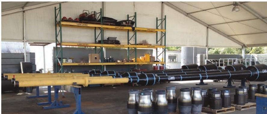
Titanium stress joint assemblies prior to installation on the Delta House FPS.
